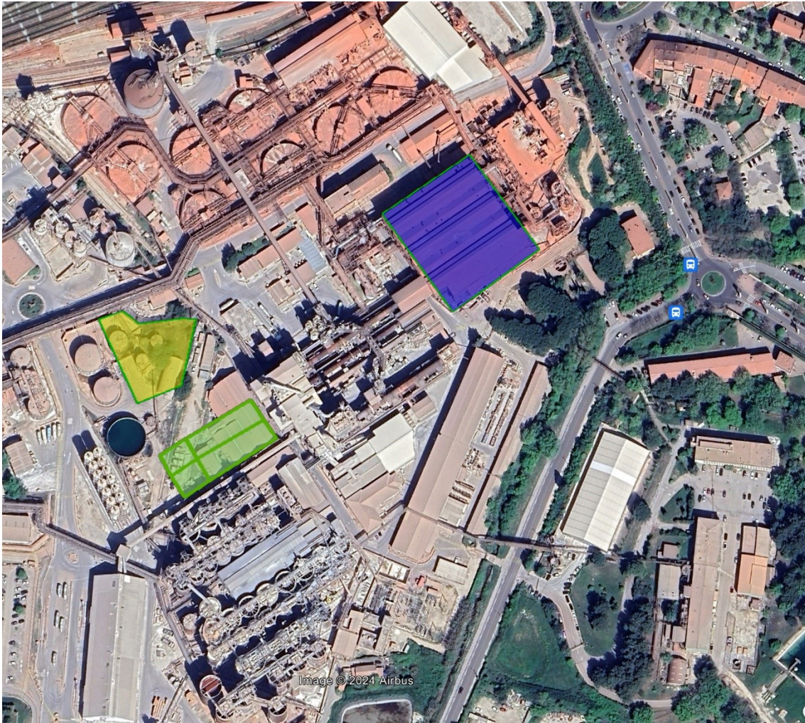
Figure 7. Location of existing digestion and future KX LTD and MVR Evaporation : Blue square: existing Digestion building (650 000 t/y Al 2 O 3 ) Green rectangle: future KX LTD building (2×100 000 t/y Al 2 O 3 ) Yellow shape : future 20 t/h MVR Evaporation section.
